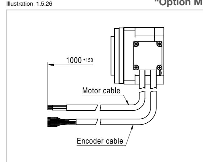
Motor and encoder cables are not suitable for moving routing!
