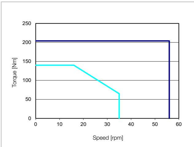
The performance curves shown are valid for the specified ambient temperature (operation) and the specified motor terminal voltage  $U_M$ .
