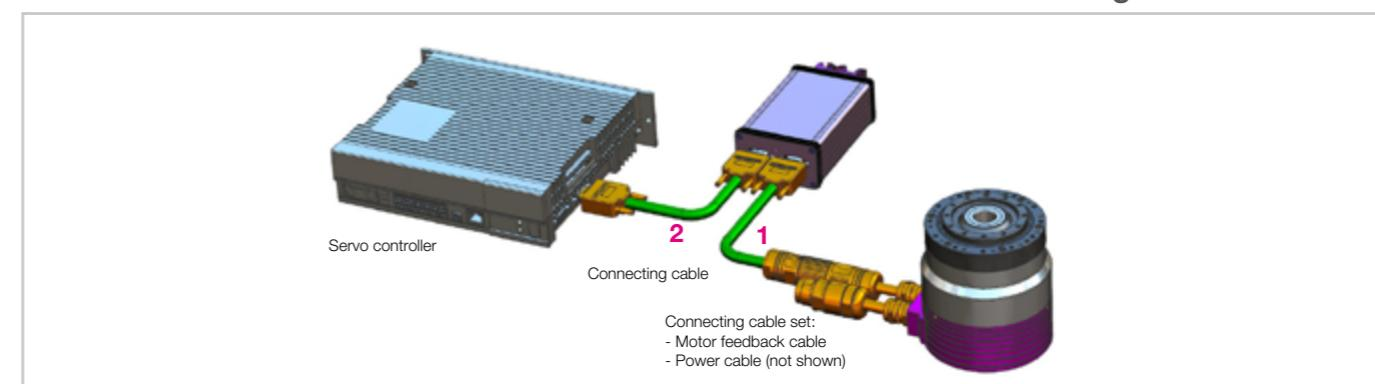
Wiring motor feedback
