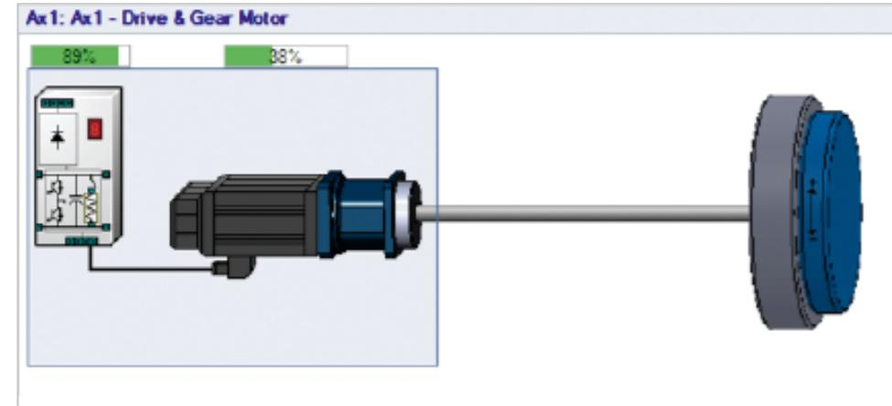
The calculation with SERVOsoft® ensures that all components are correctly designed with regard to mechanical load, and also all electrical data. For this purpose, a database was created with all relevant data of our gearboxes, motors, servo actuators and controllers.
