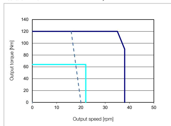
Intermittent duty — Continuous duty — Limit speed reduction with 24 VDC bus voltage - - -
