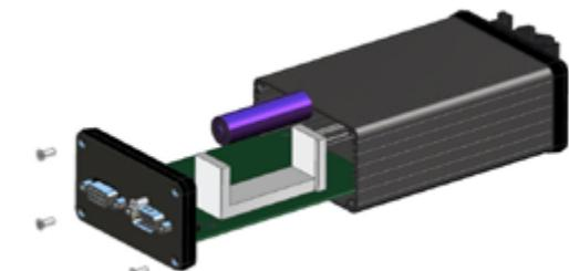
The motor feedback systems MZB, MHS and MZE monitor the connected battery and, in addition to the position values, also provide status information of the connected battery via the communication interface.
