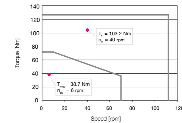
Calculation of the rms torque
