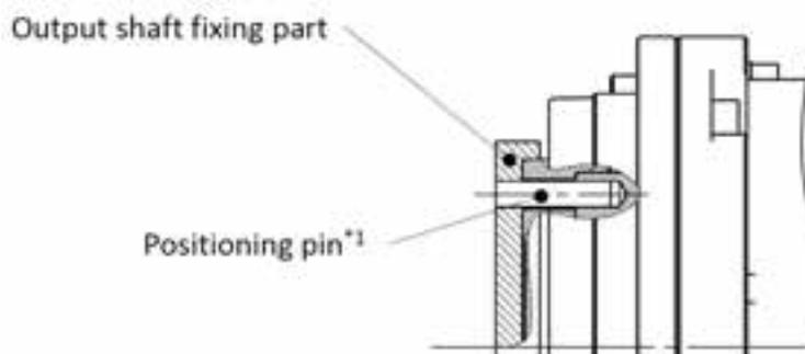
Example of use of positioning pins
