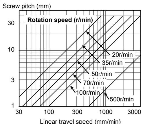
Select an appropriate reduction ratio from 8, 9, 50 and 100 so that the calculated rotation speed does not exceed the maximum rotational speed of the FLA series actuator.
