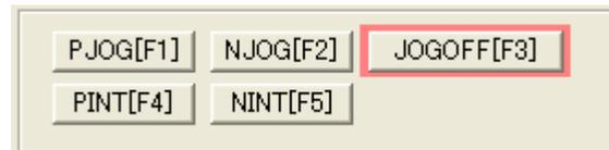
You can perform JOG operation by turning on the "CN2-7 Servo on: S-ON" signal and pressing the desired operation button.
